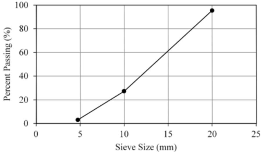
Graph.1: Size distribution curve for coarse aggregate
