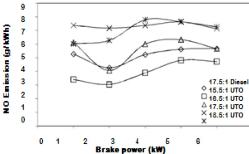
Fig. Variation in NO emission with brake power
