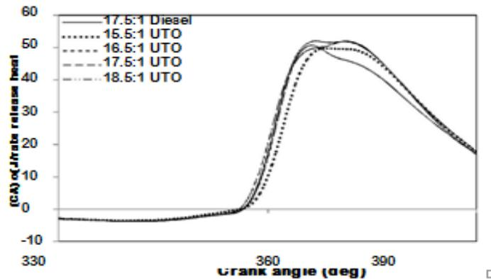
Fig. Variation of heat release rate with crank angle at full load
