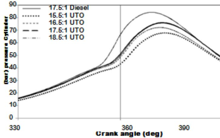
Fig. Variation of combustion pressure with crank angle at full load
