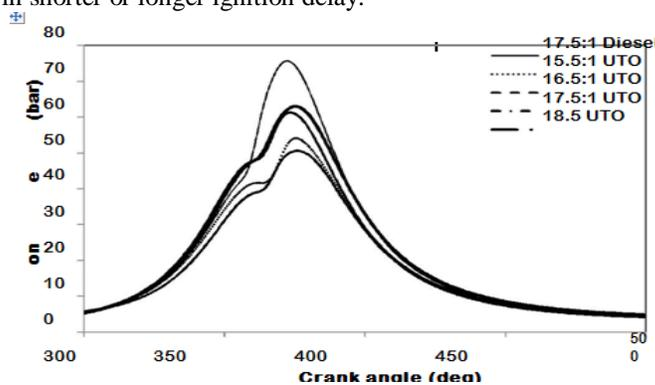
Fig. 4.1: Variation of combustion pressure with crank angle at full load
