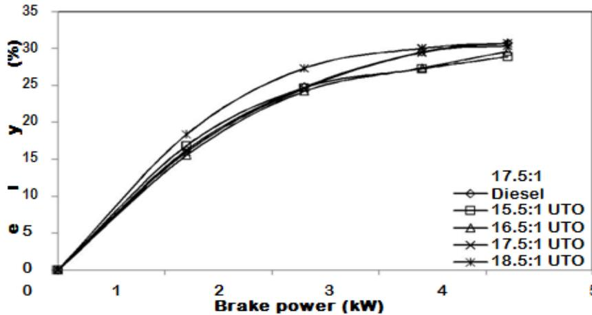
Fig. 4.4: Variation in brake thermal efficiency with brake power
