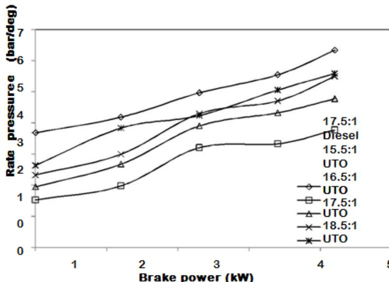
Fig. 4.3 Variation in rate of pressure rise with brake power
