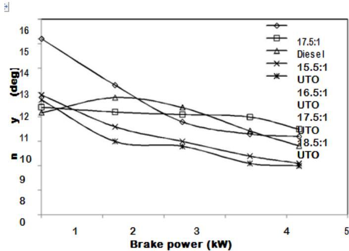
Fig. 4.2 : Variation of the ignition delay with brake power
