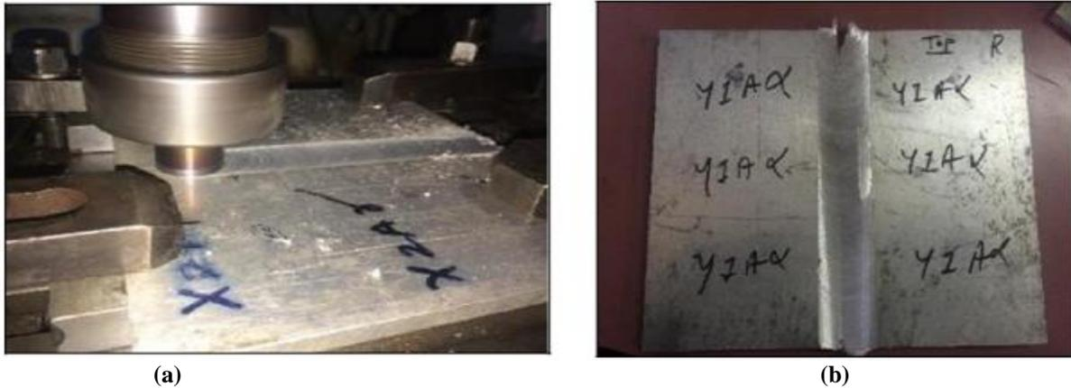
Figure 2 Tool-Base plate interaction and welded Plate
