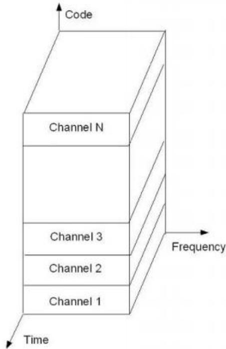
**Figure 2: The basic concept of CDMA.**
