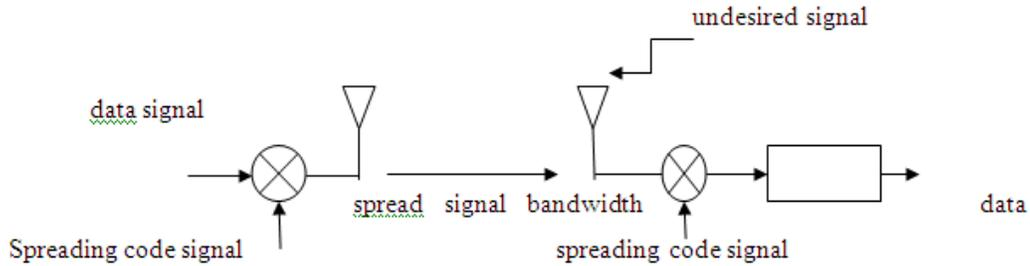
**Fig.1: Model of basic spread spectrum technique**
