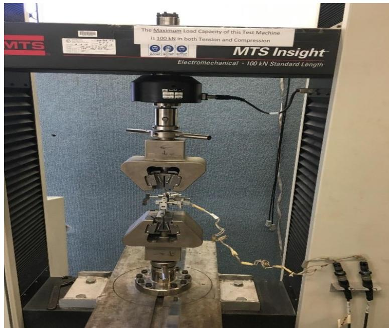
**Figure 2: Tensile testing machine**
