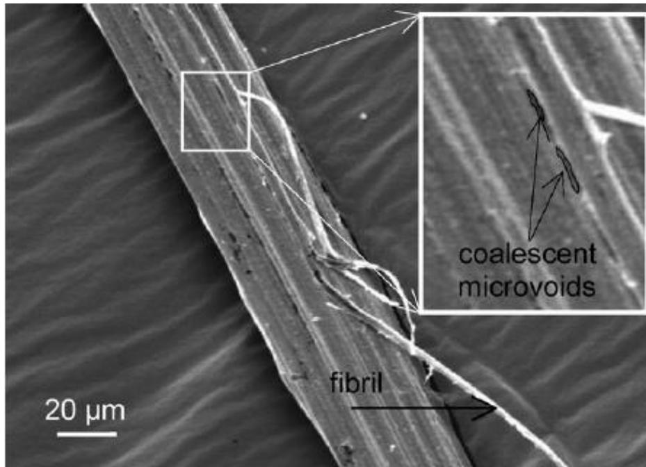
**Figure 1: SEM image of micro-voids and misaligned fibrils (Cayer-Barrioz et al. 2004)**
