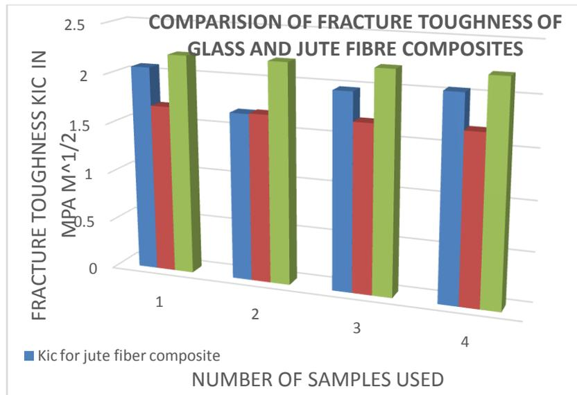
Figure 2: Comparison of fracture toughness values with GFRP made of 30 % volume fraction and different fibre lengths.
