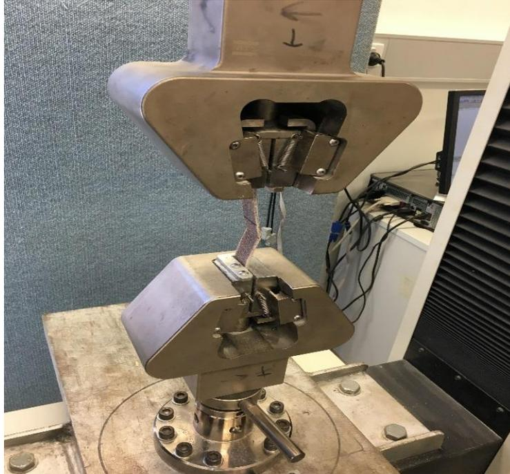
**Figure 3: Tensile testing of specimen**
