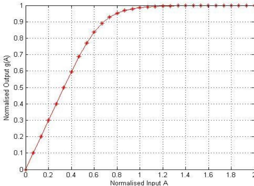
**Fig. 1.2 Input–output relation curve showing non linearity when  $p=3$ .**
