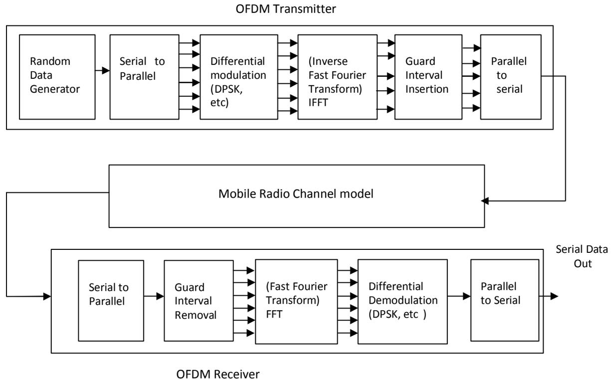
**Fig 1.1 OFDM model used for simulation**
