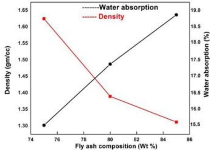
Figure.3: Water absorption and density as a function of FLY ASH Composition
