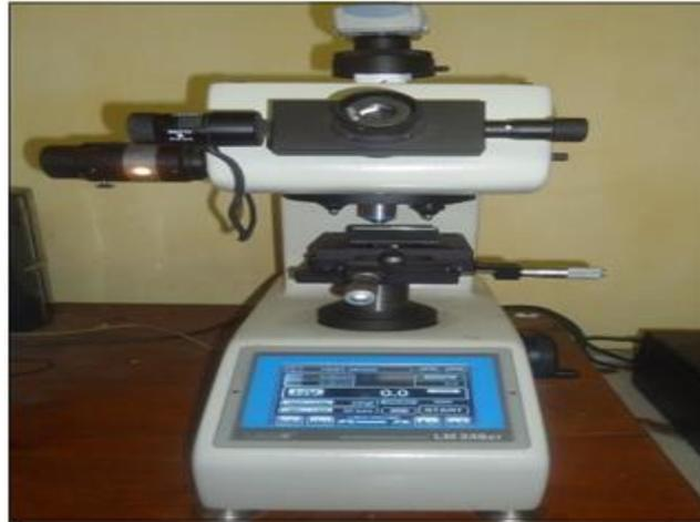
**Fig 1: Vicker hardness tester**
