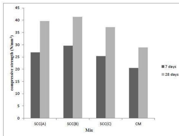
**Fig.3: Compressive strength of SCC mixes at various ages with Silica fume.**
