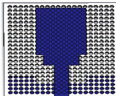
Figure 1. Configuration of the proposed microstrip-fed monopole antenna with photonic crystal as substrate ( $r/a=0.4, r=0.3, a=0.75$ ). (front view)
