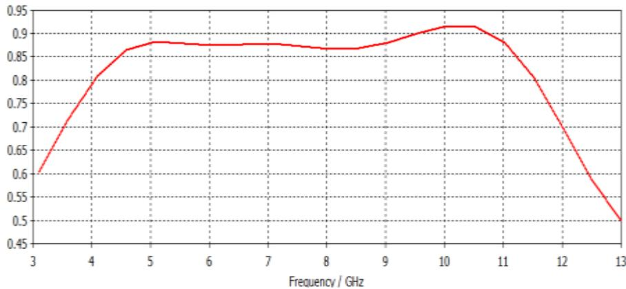
Figure 6: Gain Response of proposed antenna configuration
