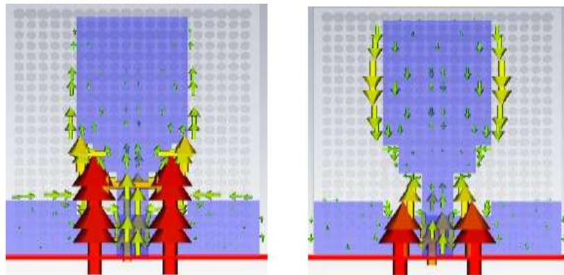
Figure 5. Simulated surface current distributions on the radiating patch for the proposed antenna shown in Fig. 1 at (a) 3.6 GHz (first notch frequency) and (b) 10.2 GHz (second notch frequency).
