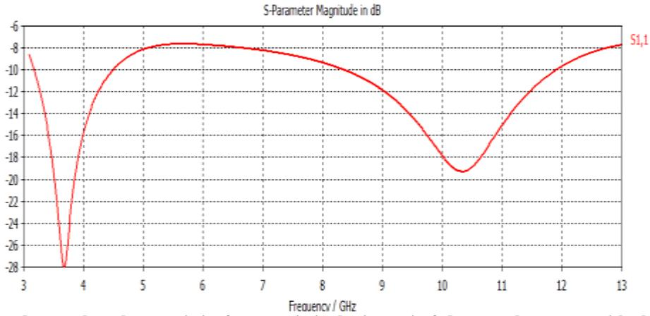
Figure 3. Simulated return loss characteristics for an optimized microstrip-fed monopole antenna with photonic crystal as substrate ( $r/a=..5$ ,  $r=1\text{mm}$ ,  $a=2\text{mm}$ )
