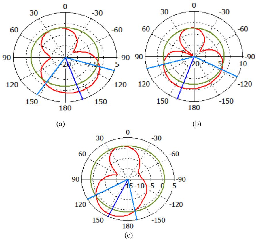
Figure 4: Measured radiation patterns of the proposed antenna. (a) 3.6 GHz. (b) 8.05 GHz. (c) 10.2GHz
