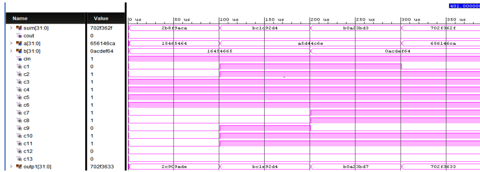
Fig.9: Simulation result of 32-bit SQR CSLA
